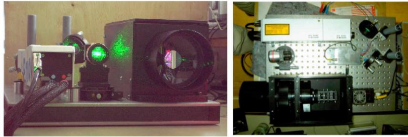
Figure 4. Hardware layout of the transponder simulation module. On the left hand side one can see the laser (from the backside), the transmit and receive aperture. The top view on the right hand side also shows the filter arrangement behind the receive aperture and the photo detection device
