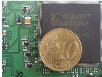
Figure 3. Prototype of the event timing hardware on the microwave link electronics.
