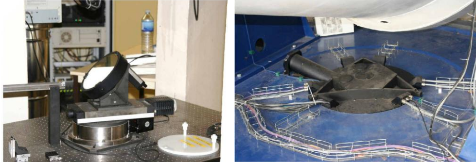
Figure 4. 200 mm high energy Fold mirrors; distribution bench on the left.
