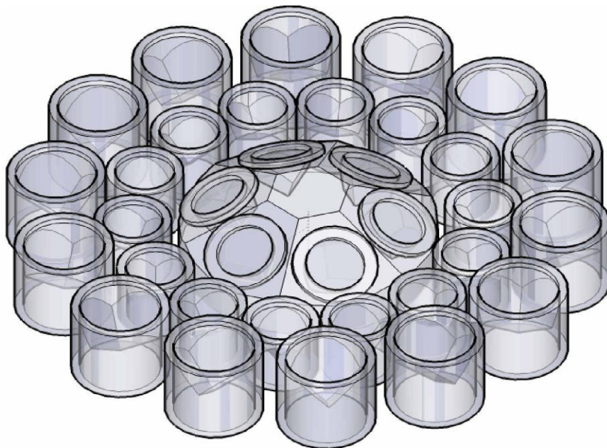
Figure 4. Basic design of ASTRO-G retroreflector array.
