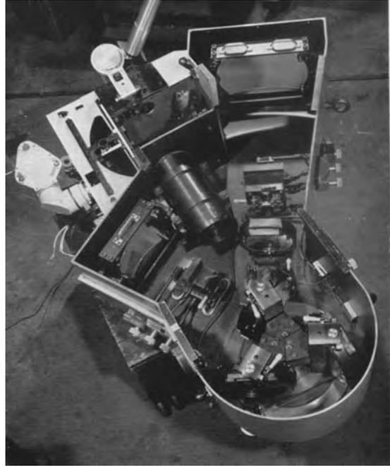
Figure 1.31. The compact Cassegrain grating spectrograph for the Mt Wilson 60-inch telescope, which was commissioned in 1956. The spectrograph had a choice of three fast Schmidt cameras, enabling faint stellar spectra to 330 nm to be recorded.
