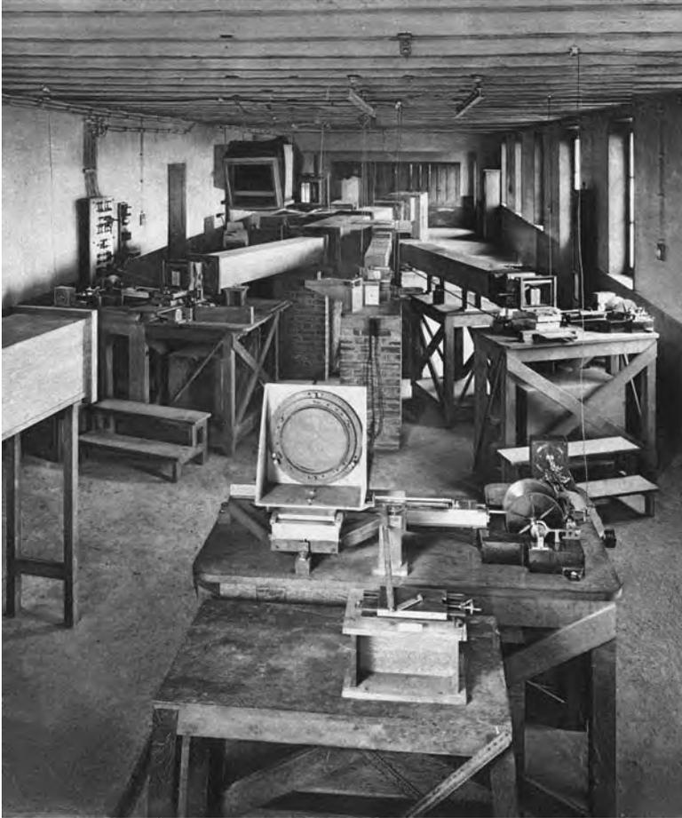
Figure 4.14. Deslandres' spectroheliograph laboratory at Meudon, 1910. Four individual spectroheliographs are united around the same astronomical objective and same collimator. The instrument on the left is the 3-m prism spectroheliograph, while that on the right is the 3-m grating instrument. Both are ready for operating.
