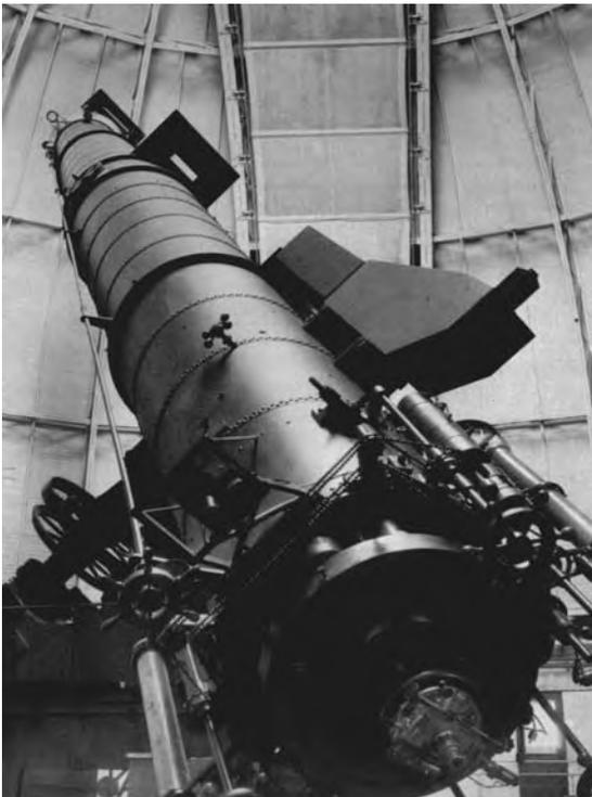
Figure 6.7. Otto Struve's ultraviolet nebular spectrograph mounted on the side of the tube of the 40-inch refractor at Yerkes Observatory, 1937.
