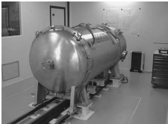
Figure 8.14. The enclosed HARPS vacuum tank, seen here in the Geneva integration laboratory prior to installation on La Silla, Chile. The tank has a volume of about  $2 \text{ m}^3$ .
