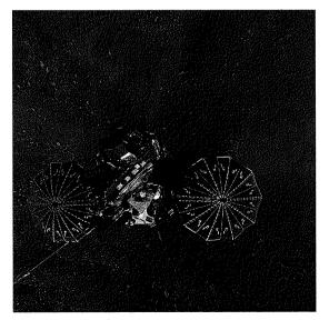
**Figure F.5** This view is a vertical projection that combines hundreds of exposures taken by the Surface Stereo Imager camera on NASA's Mars Phoenix Lander and projects them as if looking down from above. The black circle is where the camera itself is mounted. (NASA/JPL-Caltech/University of Arizona/Texas A&M, PIA11719)
